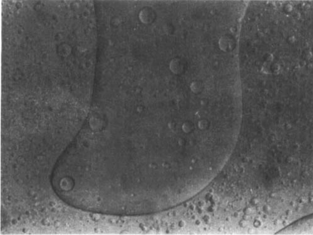
FIGURE 9 Optical micrograph of PER/HTPB (80/20) film before curing (100 \times ).
